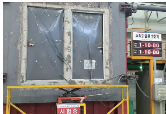
Fire resistance test of fire doors
